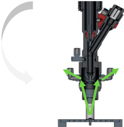
Step 3: Once tightening is complete, a vacuum system removes any dust generated during the process
