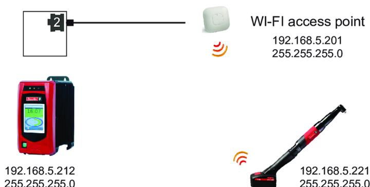
1. Connect the WI-FI access point to any Ethernet port of the controller bottom panel.
