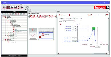
CVI CONFIG is designed to set your systems point to point or via network with an intuitive and guided interface.
