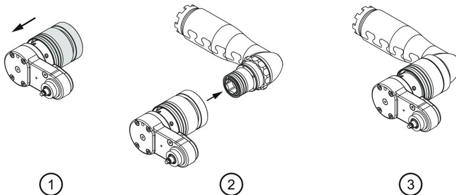
Plug an accessory into the quick-release output as shown and assign a Pset to it.
