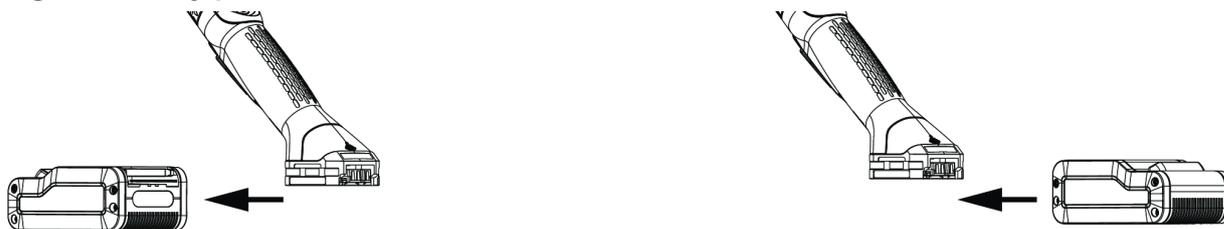
Insert the battery pack in front or behind the tool until a locking sound can be clearly heard.
