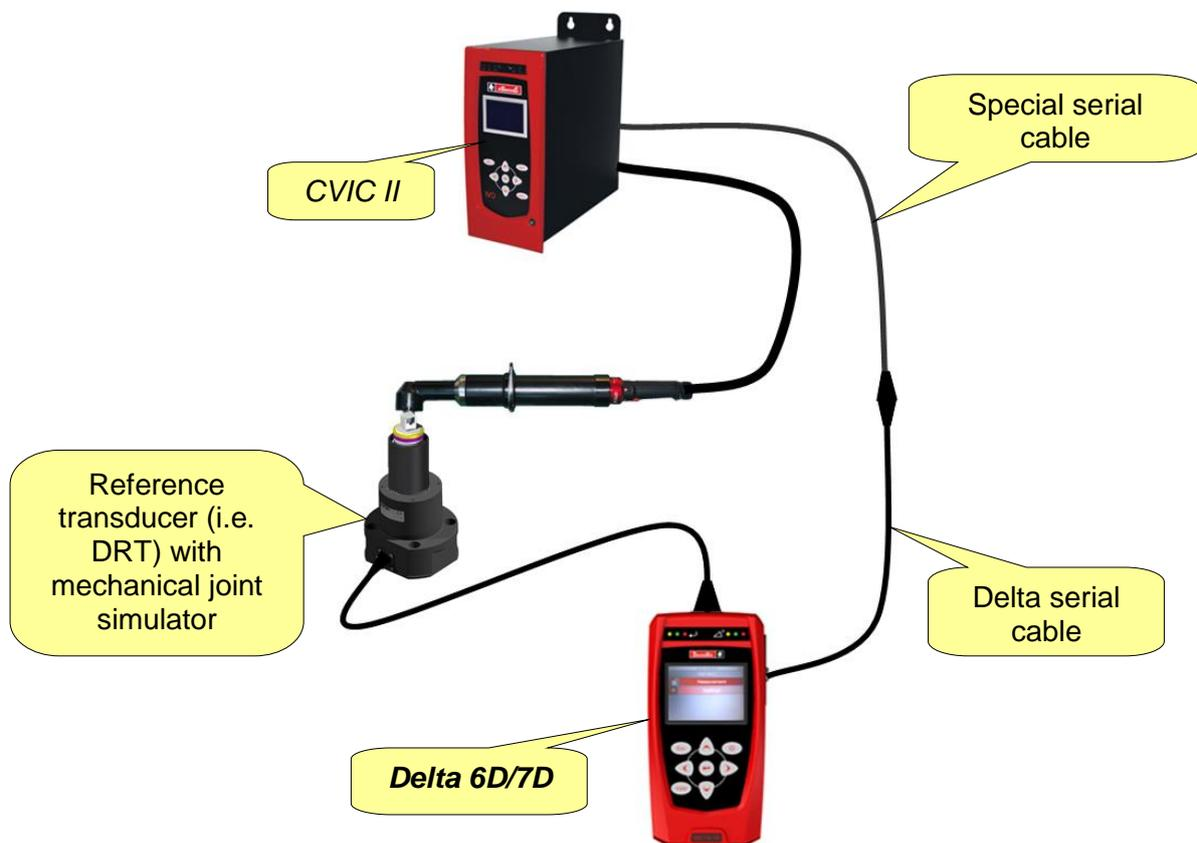
To connect the *Delta* and the *CVIC II*, use the same cable to connect the *Delta* to the external barcode reader, and the special serial cable available from the Desoutter Customer Center.
