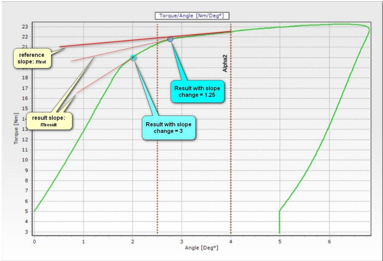
In cases like the one shown below (curve with different Breakaway and Residual points), if the algorithm doesn't find between  $\alpha_2$  and the local minimum a slope ratio surpassing the slope change set, then the result will be always taken in that local minimum.
