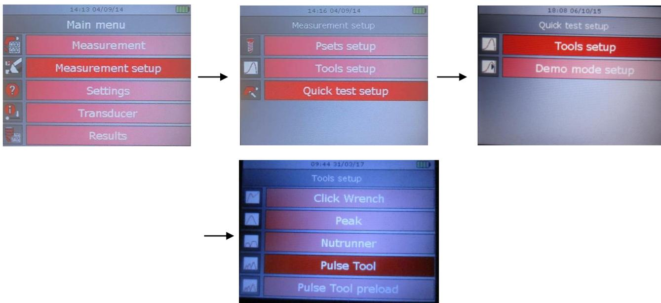
**Delta 6D/7D - Quick Test Setup**
