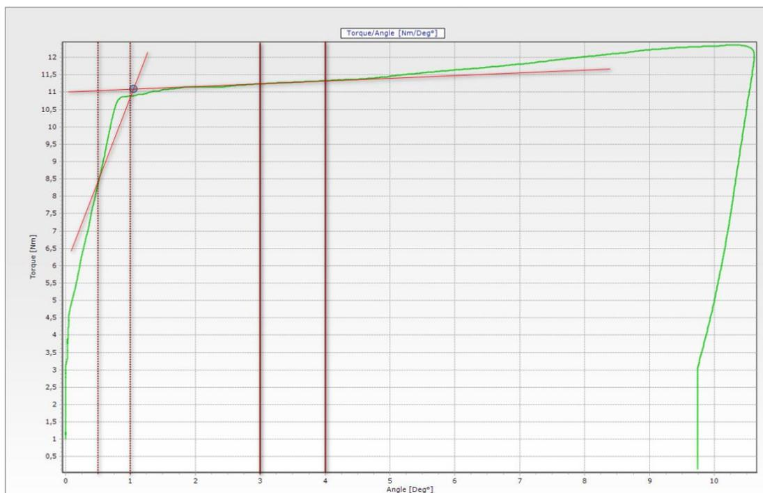
Angle thresholds:  $\alpha_1 = 0.5^\circ$      $\alpha_2 = 1^\circ$      $\alpha_3 = 3^\circ$      $\alpha_4 = 4^\circ$
