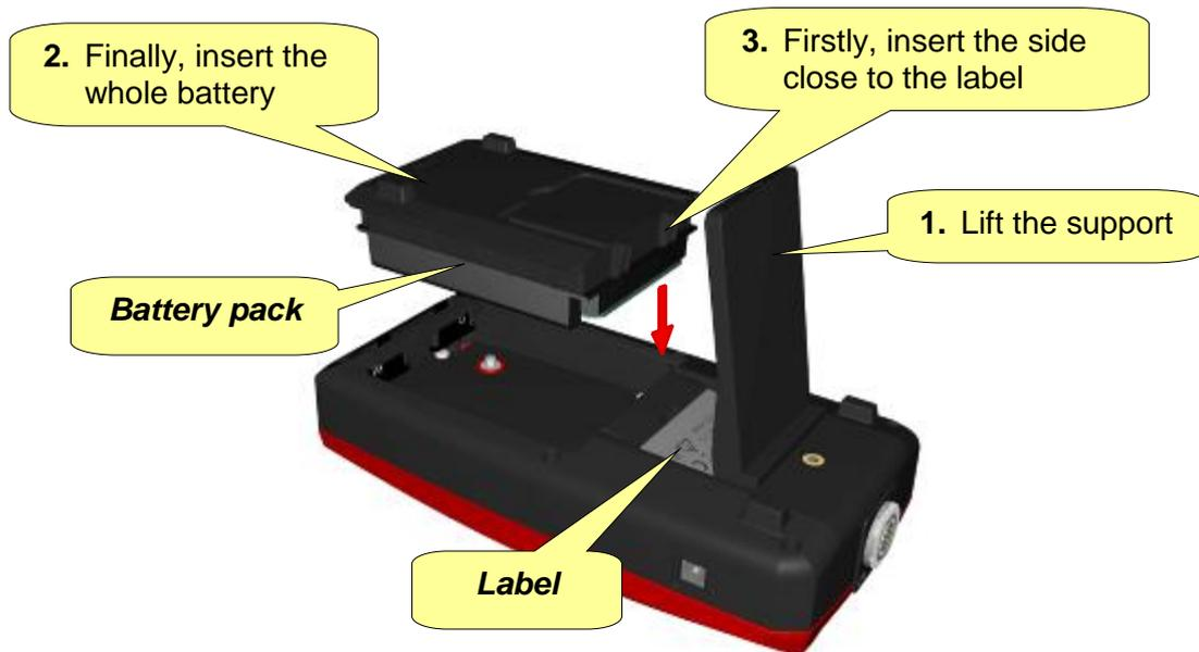
To install the battery into the Delta, turn off the Delta and install the battery, following the above instructions.
