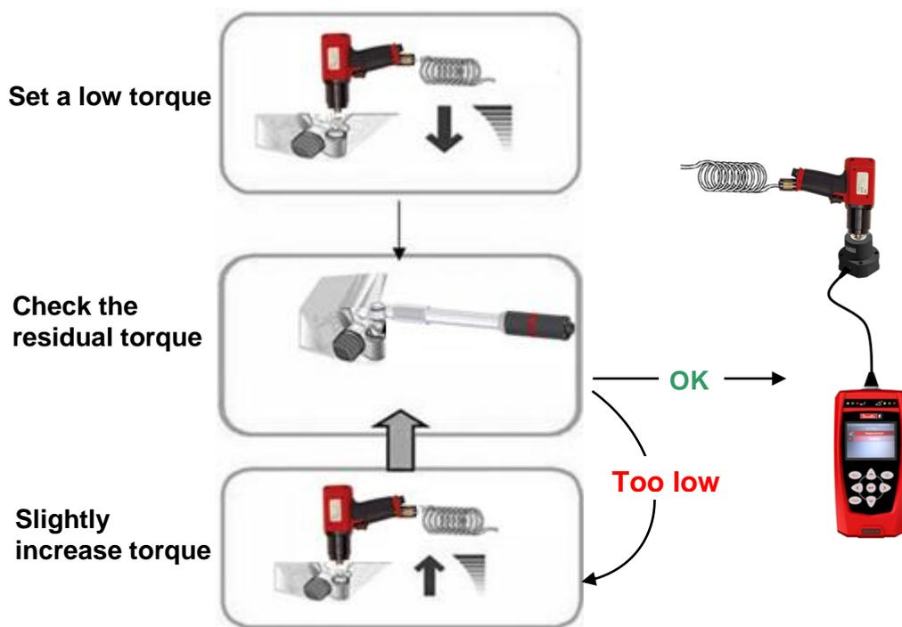
For instance, consider a target torque for the joint equal to 100 Nm. Once the tool regulation is made, the residual torque check is equal to 100 Nm.
