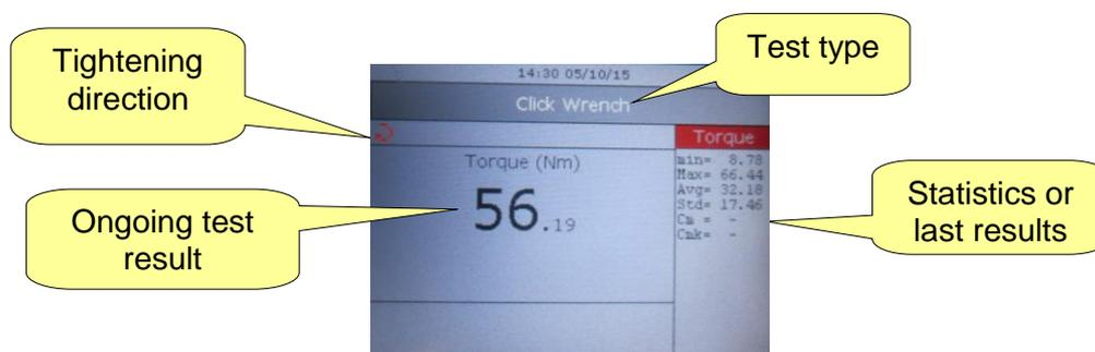
If the *Results View mode* is set to “*Last results*” in the “**Controller** → **Configuration**” menu (Delta QC software), the torque result and angle result values are shown in real time (red color for Not OK result, black color for OK results).
