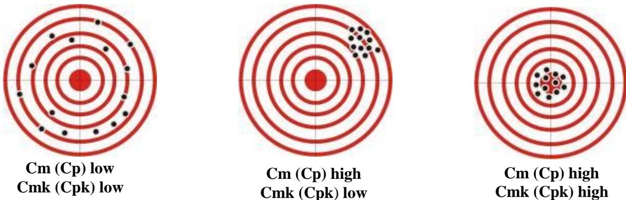
The Cm calculation depends from the tolerance limits: if the tolerance is high, the Cm value increases.
