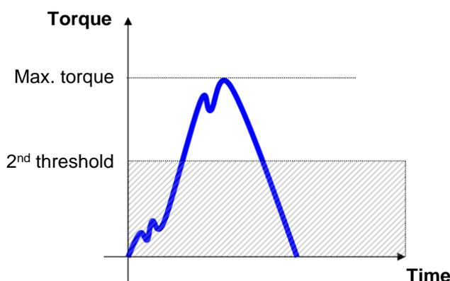
The "**2<sup>nd</sup> threshold**" is used to exclude all the part of the curve below a certain value from the analysis, where false click may occur if the operator movement is not enough steady.
