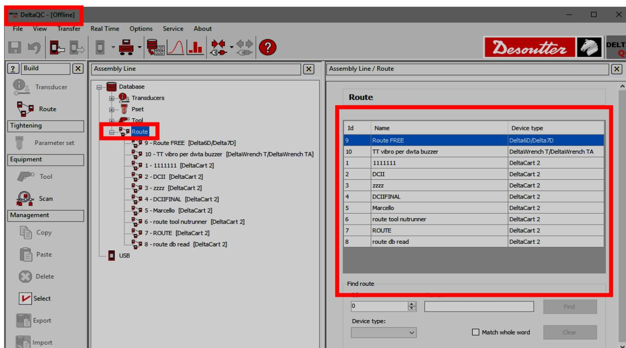
To create a new *Route*, either click on the **Route** icon placed in the *Build* area, or right-click on the **Route** node in the *Assembly Line* area (and then, select on “**Create a new Route...**”):
