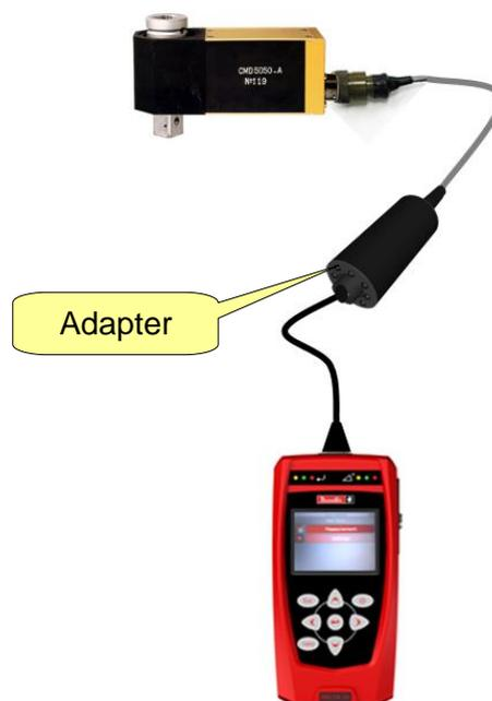
The analog transducer can be defined offline (refer to the following screen) and then transferred to the Delta, or directly online on the Delta:
