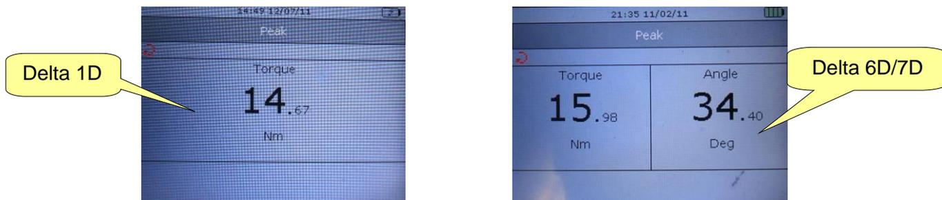
A new cycle starts when the applied torque is released, and applied again. By clicking on the **Enter** button on the keyboard the torque value is reset. The torque must be applied in the clockwise direction.
