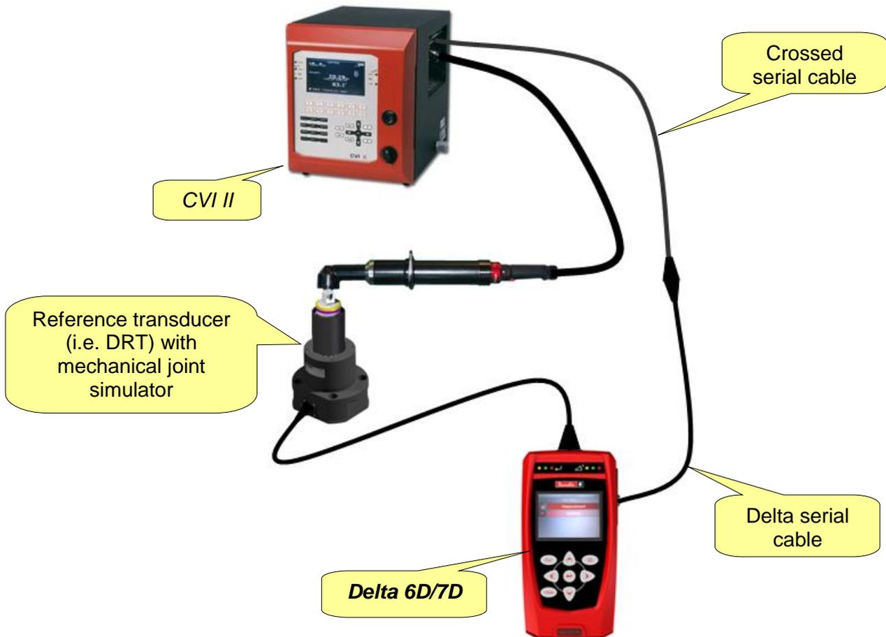
To connect the *Delta* and the *CVI II*, use the same cable to connect the *Delta* to the barcode reader, and a crossed serial cable to be connected to the serial port of the *CVI II*.
