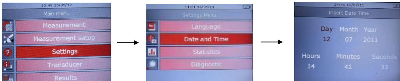
Use the **Left** and **Right** arrows on the keyboard to move in the menu, and the **Up** and **Down** arrows to increase and decrease the selected field.
