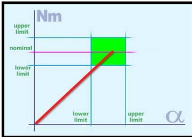
This is a more accurate method to tighten: in fact, additional information (angle) are used during the tightening process. By means of this method you it is possible to detect possible problems on the joint (refer to the following list).
