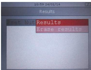
For *Tools* only, an additional menu is shown to select the *Tool*, before selecting the *Pset* associated. Select **Results** (select **Erase results** to delete the results associated with the *Tool* selected). Press **Valid** to continue:
