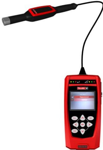
The **Quality Test on Joints** is applicable only for the **Delta 7D**. The **Delta 7D** model provides a set of test strategies to evaluate the residual torque on a joint already tighten.
