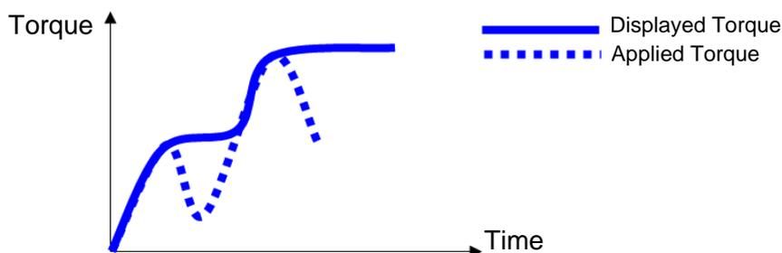
Generally, the Delta displays torque in real time (the **Delta 6D/7D** shows the angle as well), and the torque peak value is frozen on the display; the angle value is not frozen with the torque peak.
