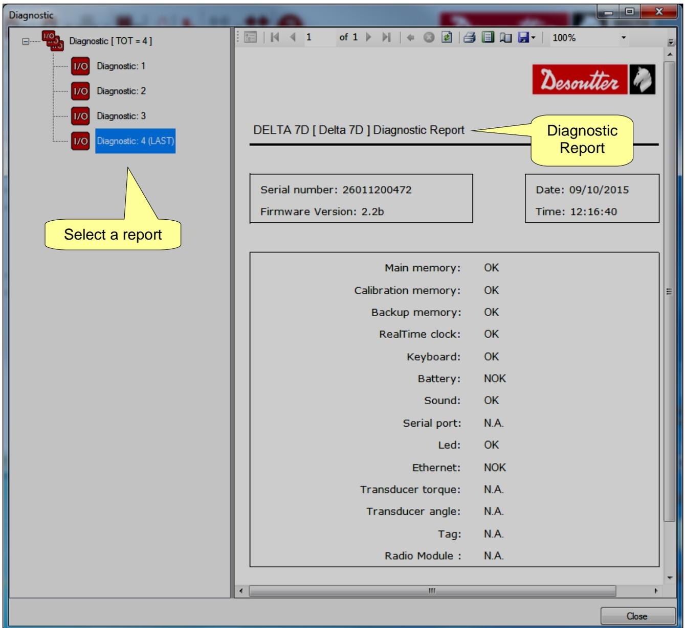
Each report is marked (in the left column) either in green if all of the test are OK (or not applicable or in red if at least one test gives a *Not OK* result.
