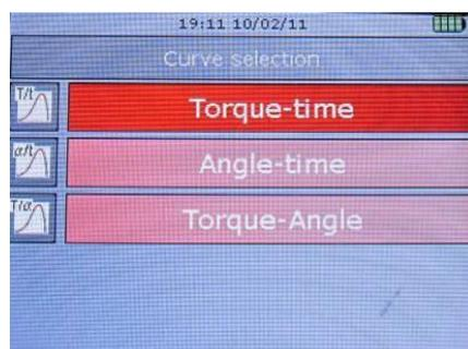
Select between **Torque-Time**, **Angle-Time** or **Torque-Angle** option.
