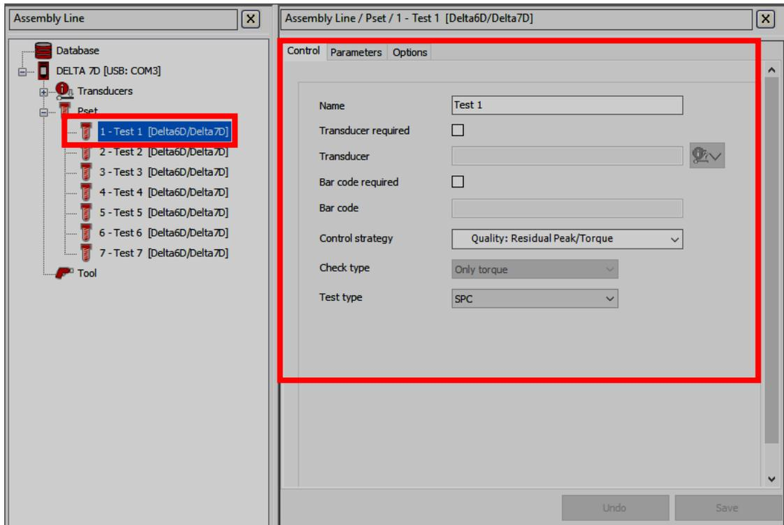
To create a new *Pset*, either click on the **Parameter set** icon placed in the *Build area*, or right-click on **Pset** in the *Assembly Line* area (and then, click on **Create a new Pset...**):
