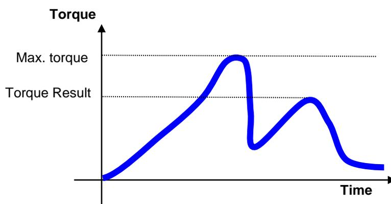
A typical scenario can be represented by the search of the last torque in self-tapping or special screws, where the last torque peak is considered the torque applied to the joint.
