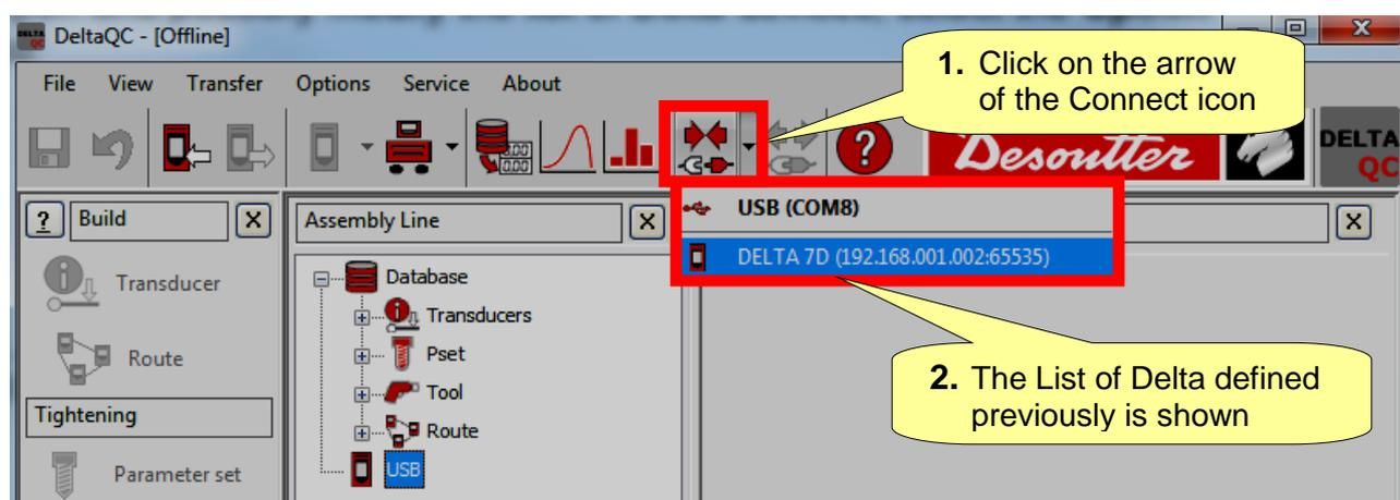
Connect the network cable to the Delta and select it from the list.
