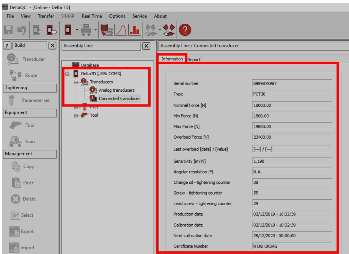
The additional field **Last overload** indicates the date, time, and value of the last overload detected by the Delta.
