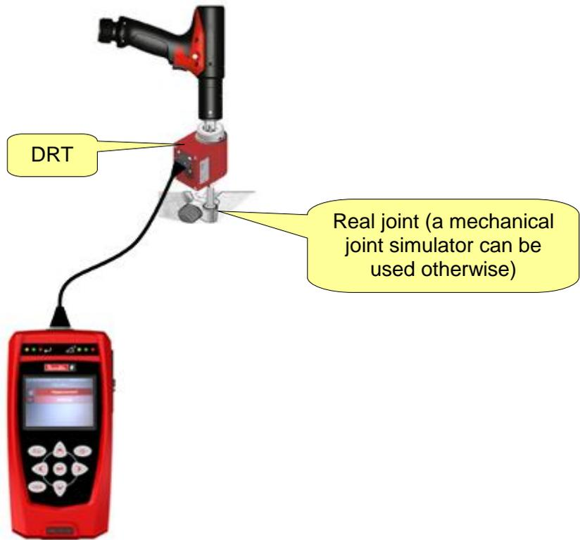
A DRT on the real joint (or a mechanical joint simulator) can be used. This also provides the angle measurement:
