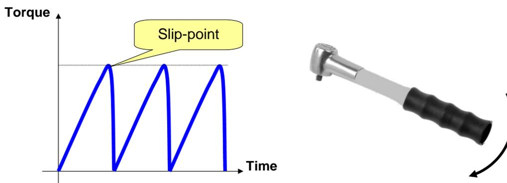
The torque result is the peak value measured during the test.
