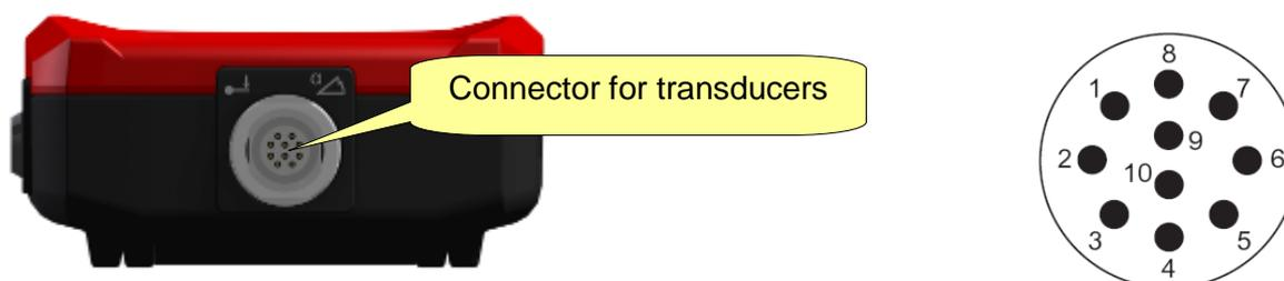
The ten pins connector is available to connect the transducers to the Delta.
