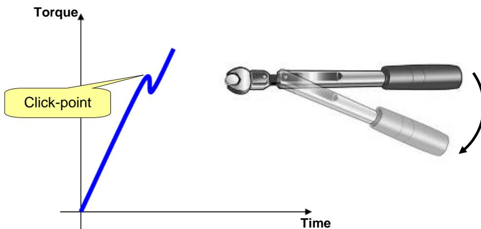
The click-point is detected when the torque drops down and then increases again, producing the typical shape of the “click” phenomenon (refer to the following examples):
