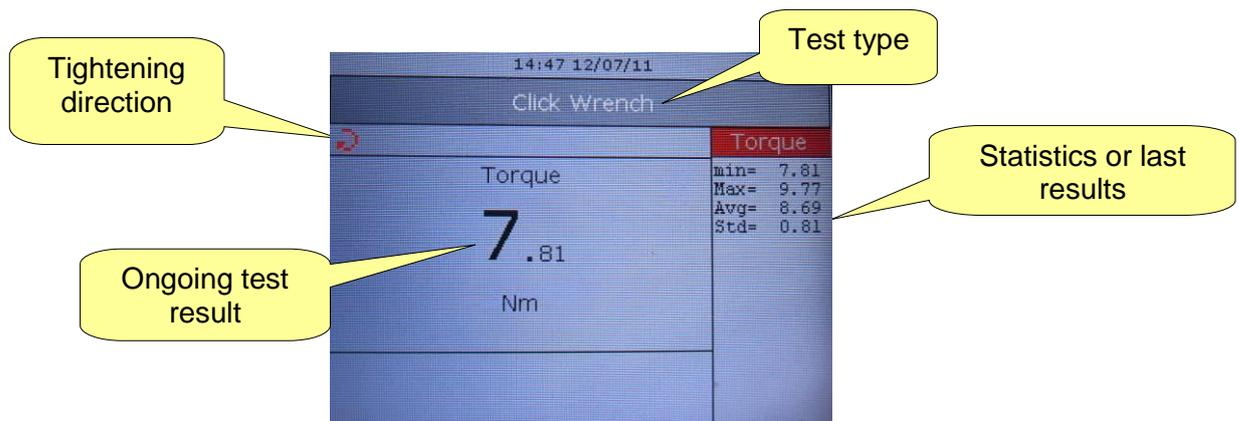
If the *Results View mode* is set to “*Last results*” in the “**Controller** → **Configuration**” menu (Delta QC software), the torque result and angle result values are shown instead of the statistics (red color for Not OK result, black color for OK results).
