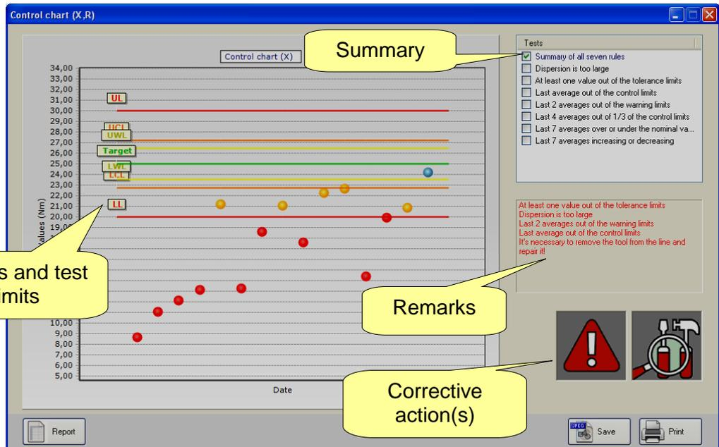
The summary shows all of the results with the test target and limits values (note that if a set of tests was performed in a Cm-Cmk test having batch number over ten, only the last ten results of that batch are considered).
