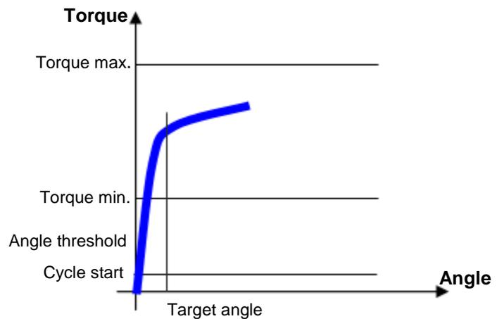
Define the **torque limits** for considering as OK the test result.
