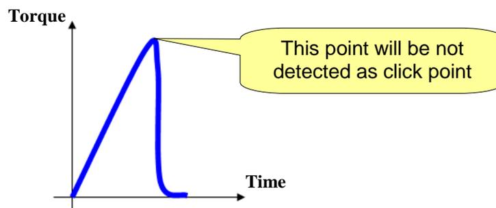
If the test ends and the click-point is not detected, the message “**not detected**” is shown on the display. In this case, the result is the “*torque absolute peak*”.
