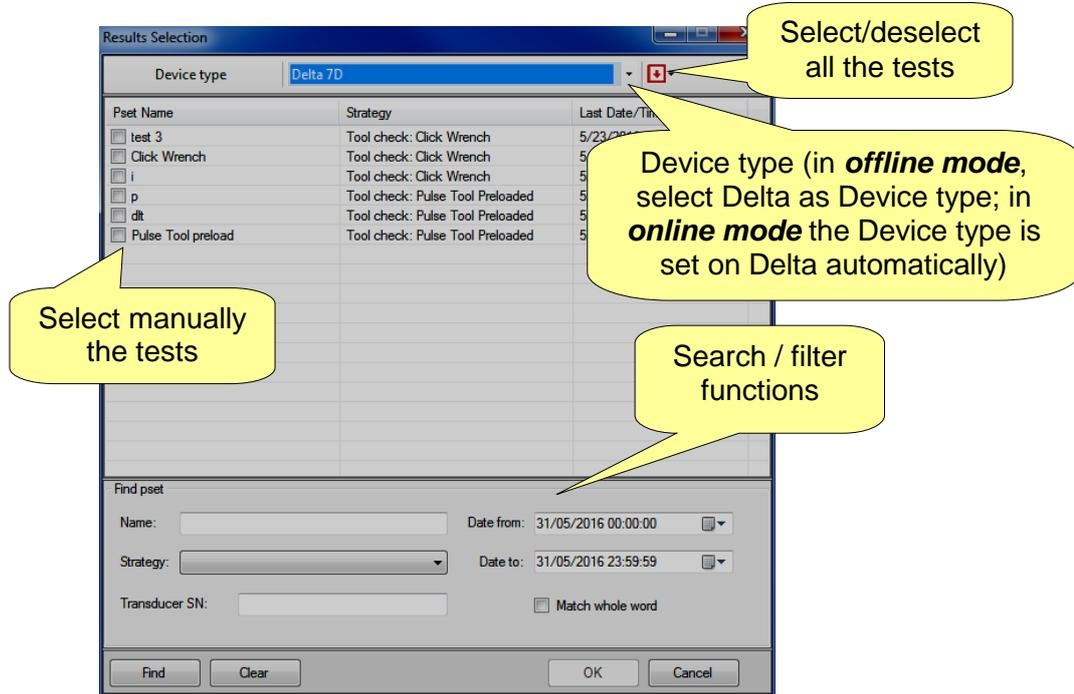
Select the **Device type** (when working *offline*, otherwise the instrument connected is automatically selected) and the tests to be reviewed. Finally click on **OK**.
