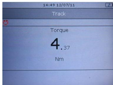
Torque can be applied in either clockwise (positive torque) or counterclockwise (negative torque) direction.
