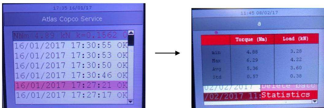
In the same way, both torque and load values are shown into Batch Results screen.
