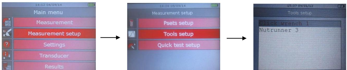
Press the **Enter** button on the Delta keyboard to *Modify/Delete* the selected *Tool* (press **Valid** to confirm), or to create a new one:
