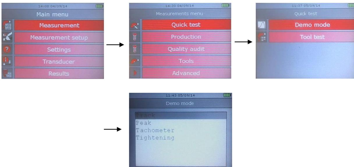
Select **Track**, **Peak**, **Tachometer** or **Tightening** and click on the **Enter** button on the keyboard to start the test.
