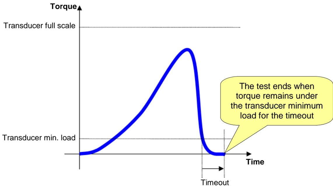
For two-steps tools, the “**Timeout**” allows the tool to switch between the two steps without ending the test.
