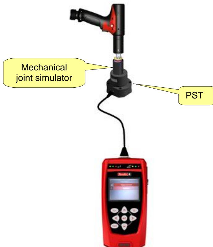
During the test, the torque result (and the angle for **Delta 6D/7D**) is displayed:
