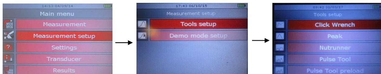
**Delta 1D – Quick Test Setup**
