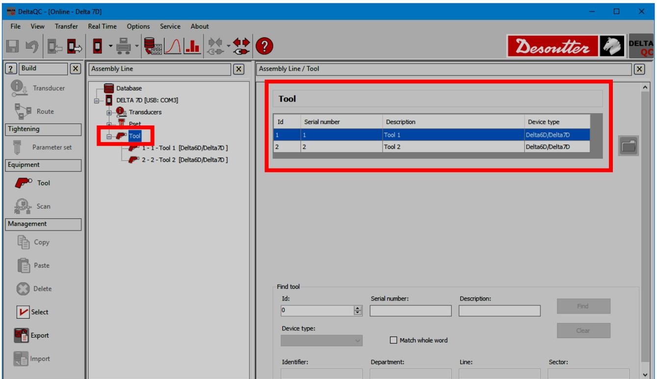
Select a *Tool* from the *Assembly Line* area to display its parameters:
