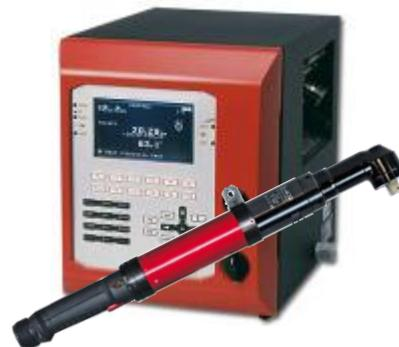
For *Nutrunner Test*, the torque result shown by the *Delta* is the peak value measured during the test.
