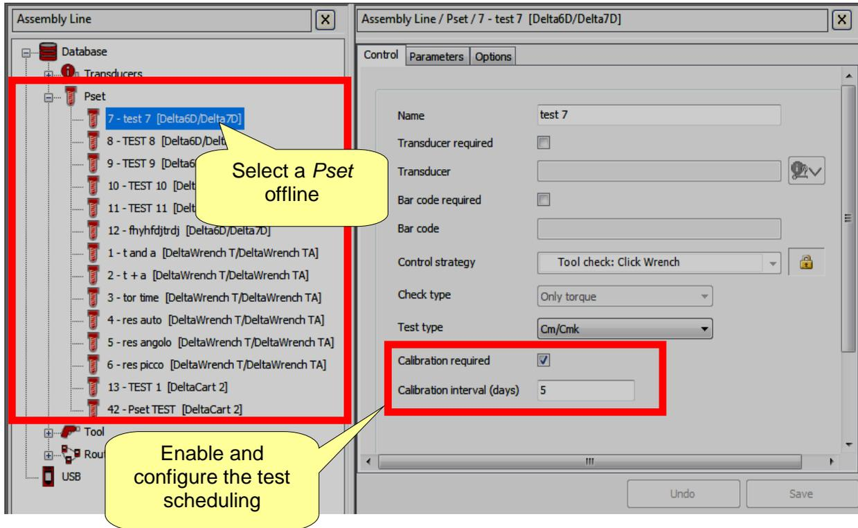
After linking the *Tool(s)* to the relative *Pset*, select **Pset** in the **Assembly Line** area:
