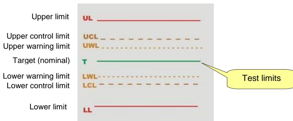
*Upper Limit* (UL) and *Lower Limit* (LL) are the test limits specified for the test. The other limits are calculated as follows:
