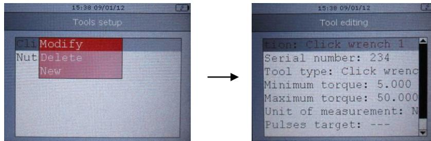
Scroll the parameters using the **Up/Down** keys and click on **Enter** to edit the parameter selected. Then set the value by means of the arrow buttons (left/right to select the digit, up/down to increase/decrease the value). Finally, either click on **Valid** to save or click on **Esc** to quit without saving.
