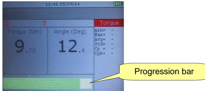
The progression bar guides the operator to the target torque.
