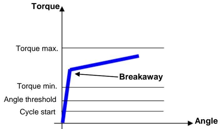
Sometimes, very high static friction is built into the joint (for instance, either for no lubrication or conical seat). In that case, as soon as the bolt moves, the torque decreases and the real residual torque is lower than the peak torque necessary to overcome the static friction:
