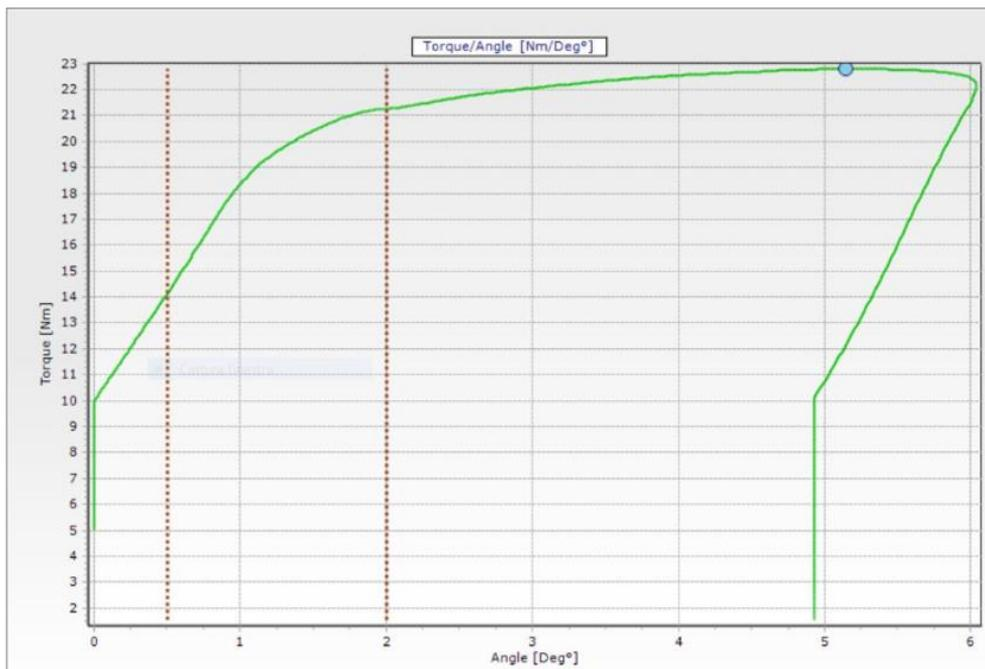
No minimum after breakaway detected → Result NOT OK and torque peak marked on the curve
