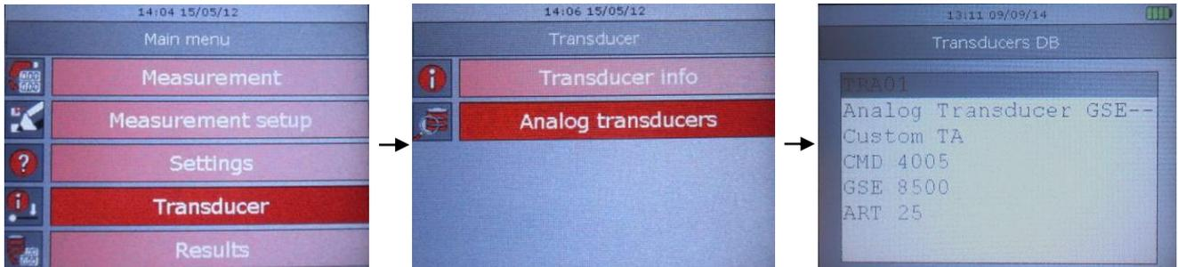
Select the transducer and press **Valid** to confirm or **ESC** to quit without selecting the transducer.
