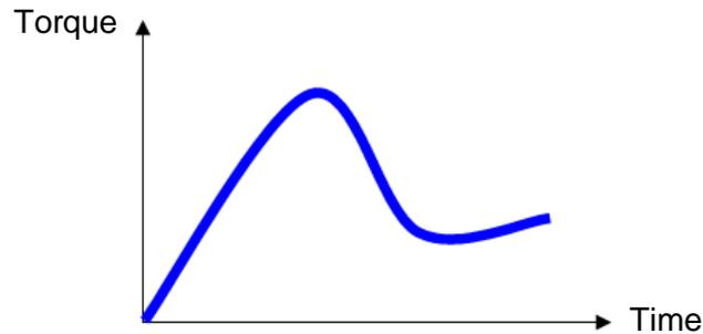
In **Track** mode, the Delta simply displays the applied torque in real time.
