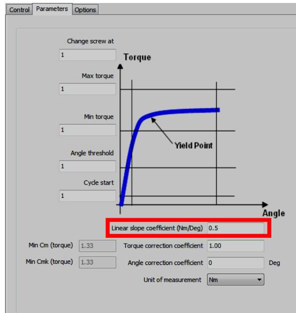
The “**Linear slope coefficient**”, that characterizes the *Yield Point control strategy*, may be calculated (for each single joint, only after executing a trial test in order to get data for calculating it) as follows:
