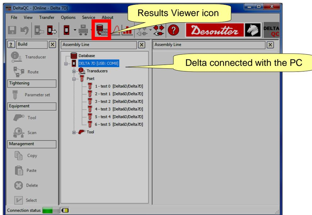
To view the results downloaded from the Delta and stored into the database, work in *Offline mode*:
