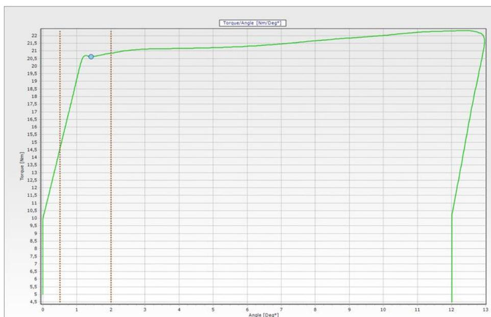
Angle thresholds set:  $\alpha_1 = 0.5^\circ$        $\alpha_2 = 2^\circ$
