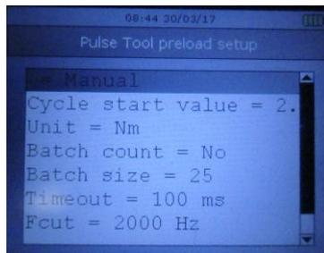
Scroll the parameters by means of the **UP/DOWN** keys; then click on **Enter** to edit.
