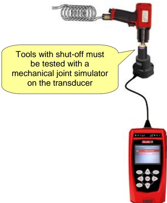
Tools with shut-off must be tested with a mechanical joint simulator on the transducer
