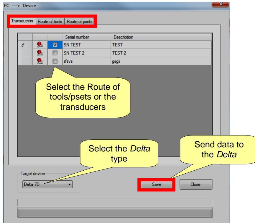
Select either the *Route of tools/psets* or the *transducers* and click on **Save** to send data to the *Delta*. It is possible to send one *Route of tools* and/or one *Route of Psets* to each *Delta*. It is also possible to transfer to the *Delta* the analog transducers defined offline.
