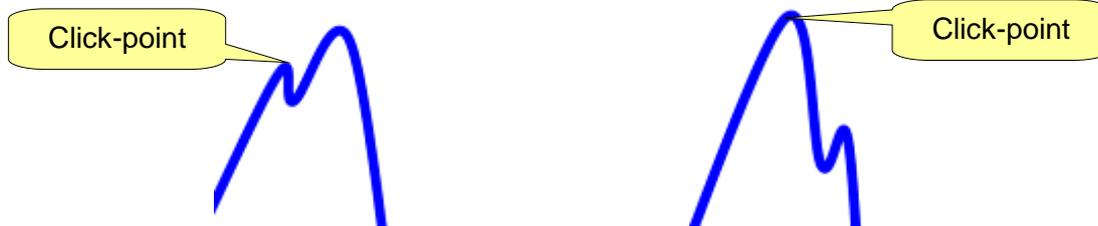
If the torque only drops down to zero (without increasing again) after a peak-point (as shown in the figure below), the click-point is not detected. For this reason, slip-wrenches cannot be tested with this method (slip-wrenches should be tested with the *Peak Test* (refer to the paragraph “*Peak Test*” for further details)):
