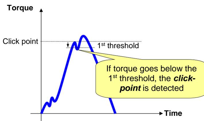
For instance, if the peak is 100Nm and the *1<sup>st</sup> threshold* is set to 10%, the torque must go under 90 Nm, in order that it can be considered the **click point**.
