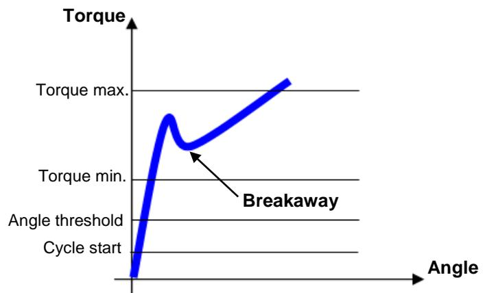
In both the above cases, the Delta algorithm detects the proper breakaway point.
