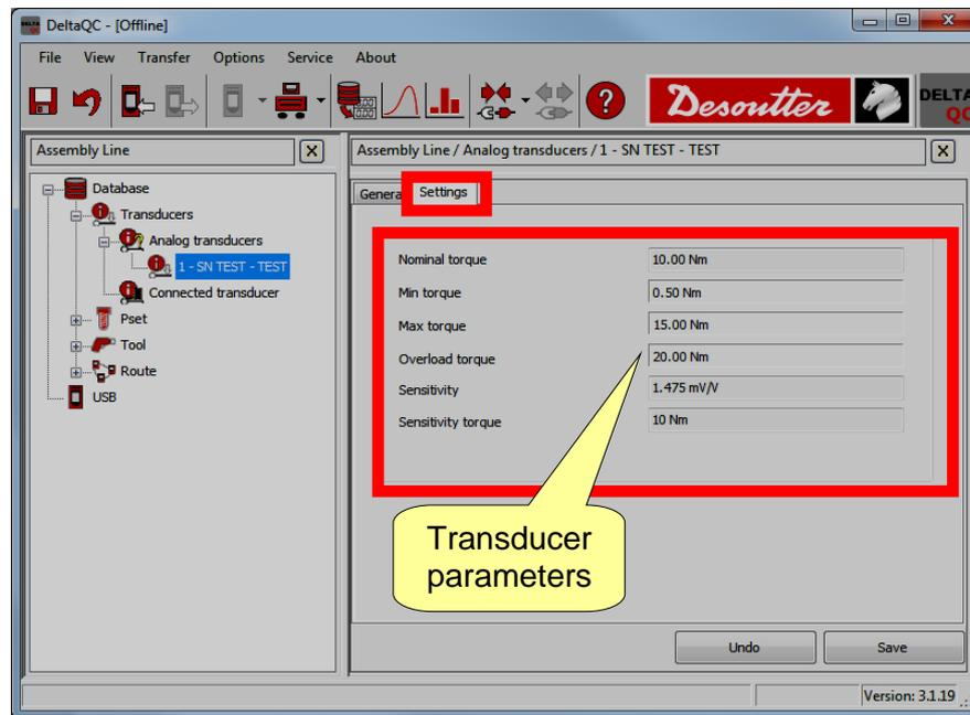
For *pre-defined transducers*, the parameters are set according to the type selected, and cannot be modified.
