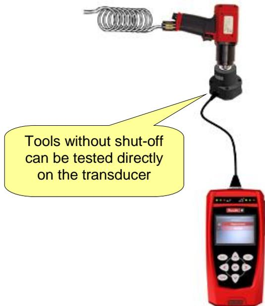
Tools without shut-off can be tested directly on the transducer
