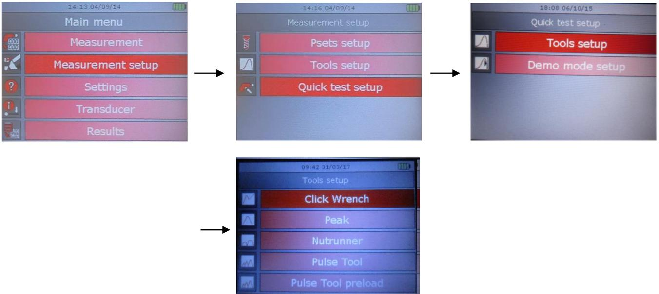
**Delta 6D/7D - Quick Test Setup**
