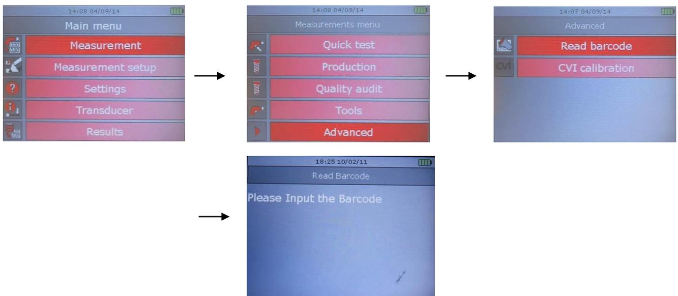
Scan the barcode string by means of the barcode reader (*integrated barcode reader or external barcode reader*) and the associated *Pset* starts automatically.
