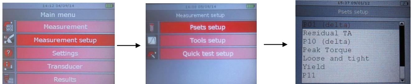
Press the **Valid** button on the Delta keyboard to **Modify/Delete** the selected *Pset*, or to create a new one:
