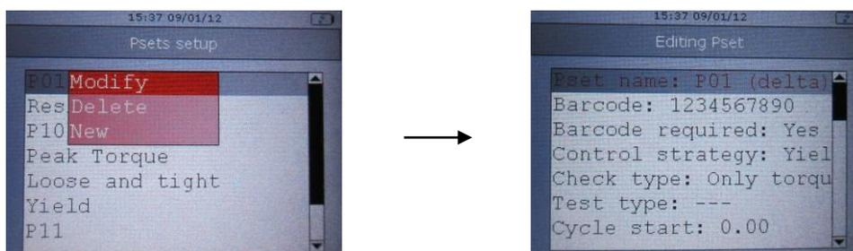
Scroll the parameters using the **Up/Down** keys and click on **Enter** to edit the parameter selected. Use the arrows on the Delta keyboard to set the value by means of the arrow buttons (left/right to select the digit, up/down to increase/decrease the value). Finally, either click on **Valid** to save or click on **Esc** to quit without saving.
