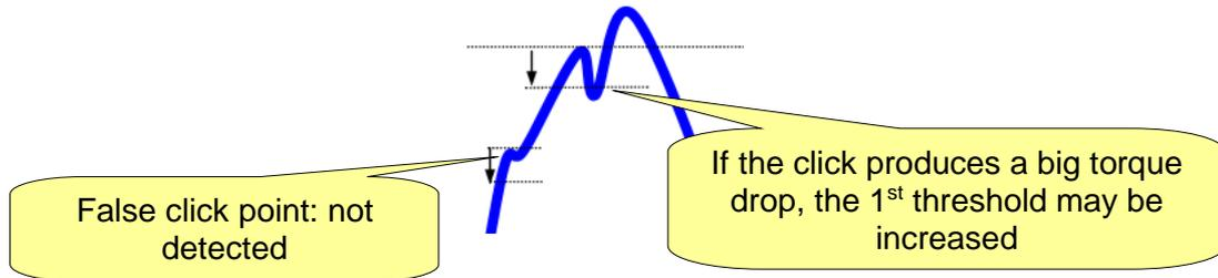
On the other side, if the **click point** produces only a little drop in the torque, this *1<sup>st</sup> threshold* may be decreased in order to detect the *click point*.
