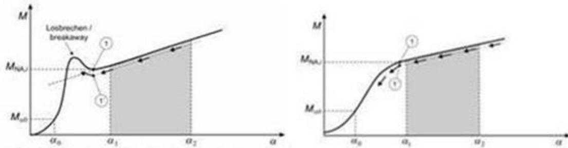
The result is expected to be OK before the angle threshold  $\alpha_1$
