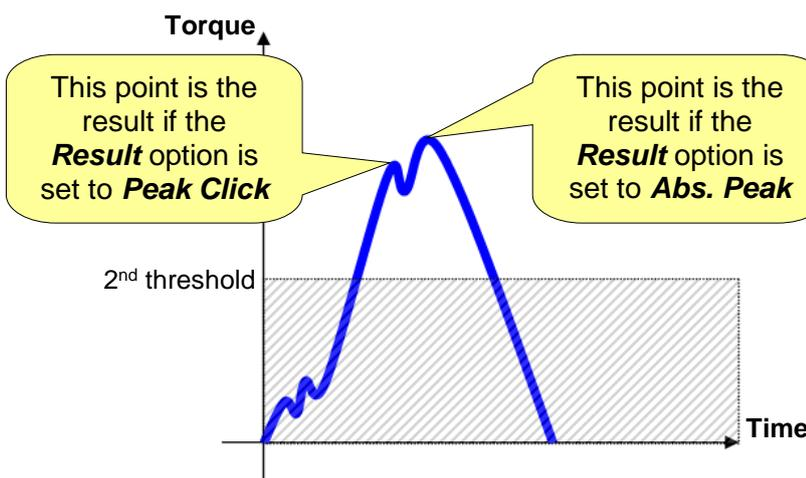
The “**Result**” defines the peak that must be taken as torque result. If the **Peak Click** is selected, the first peak (*click point*) is considered as result of the test; otherwise, if the **Abs. Peak** is selected, the maximum torque is considered as result.
