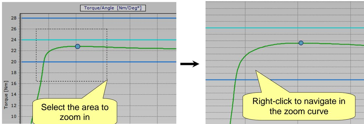
While zoom in, to navigate the graph right-click the curve and move the mouse pointer on the graph. To zoom out to the whole curve, press the left button on the mouse, move the cursor up/leftward, and release the left button:
