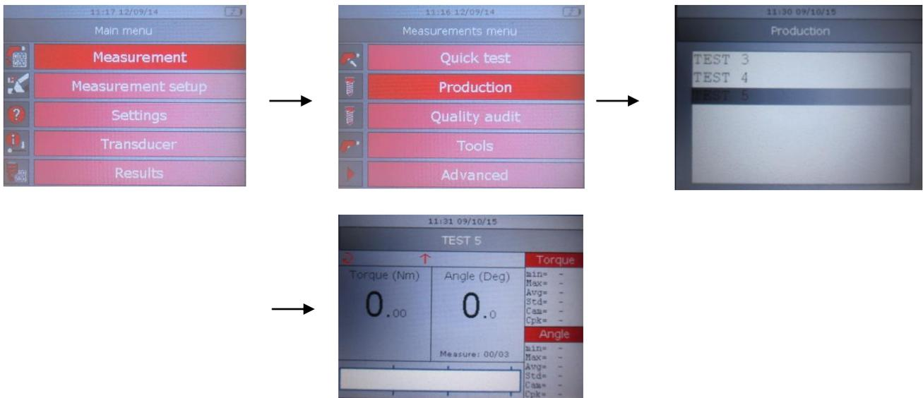
3. Apply the target torque specified in the Pset, operating the Q-AUDIT on a vise:
