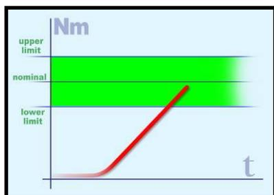
This is the easiest tightening method: it is enough to apply the torque within the limits (refer to the figure on the left).
