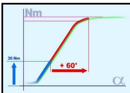
The bolt is first tightened to a certain torque and then it is further tightened to a specific angle.
