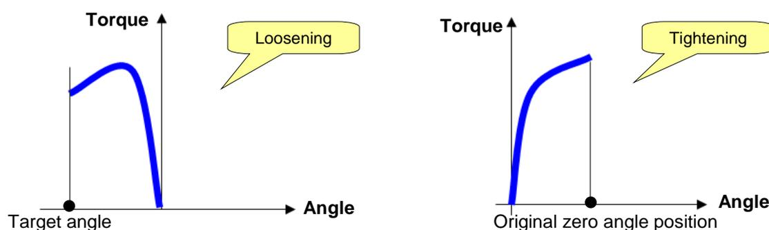
Specify the torque limits. The residual torque result is the torque at the end of the retightening operation (measured when the original zero angle position is reached back).
