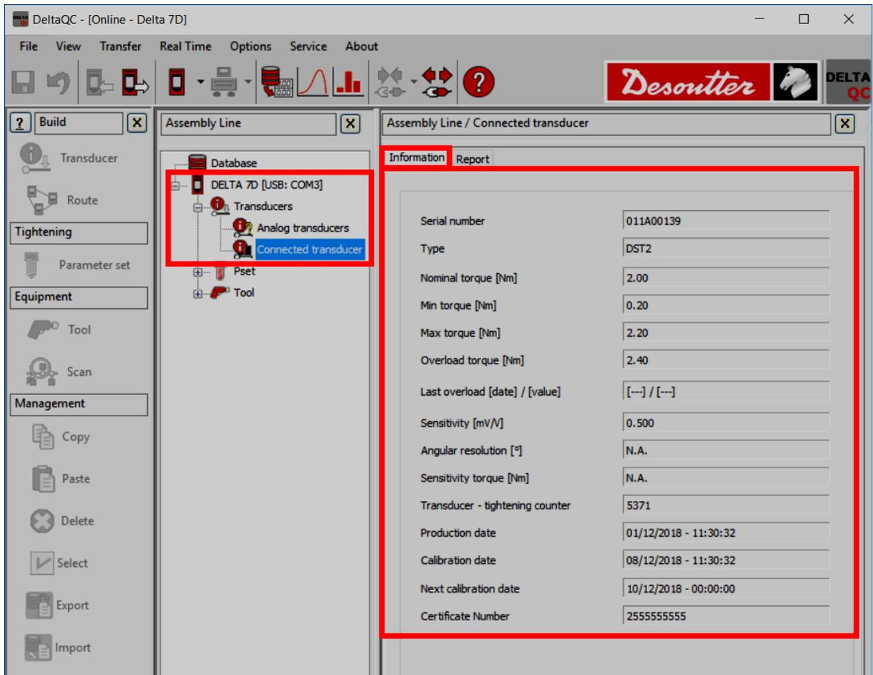
The additional information **Last overload** indicates the date, time, and value of the last overload detected by the Delta.
