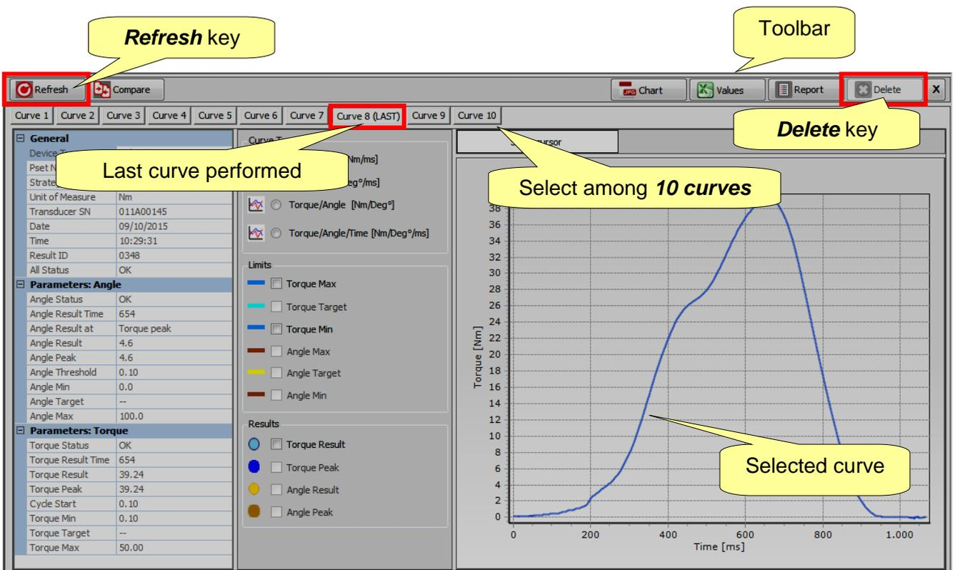
When the Delta is connected with the DeltaQC Software (**online** mode), the last curve performed can be recognized due to the “**(LAST)**” placed close to the *curve number*.
