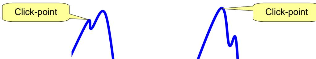
If the torque only drops down to zero (without increasing again) after a peak-point (as shown in the figure below), the click-point is not detected. For this reason, slip-wrenches cannot be tested with this method (slip-wrenches should be tested with the *peak-wrench* function):
