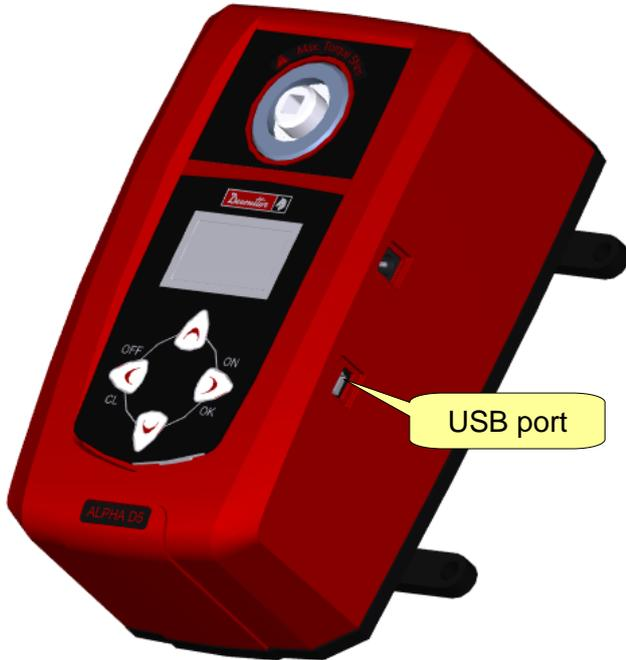
The USB port is available for programming the Alpha by means of *DeltaQC* Software.
